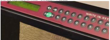
Use the arrow keys to insert a space or correct any mistakes. Once complete, press "Enter" on the keyboard. Complete your ballot. Press "CAST VOTE".
